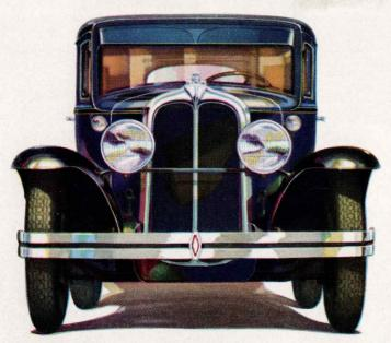
A FRONT view of the Pontiac Big Six shows the deep, chrome-plated shell of its cross-flow radiator. The distinctive vertical bar in the center of the radiator is also chrome plated, as are the headlamp rims, cowl lamps, the cowl band, and many other exposed bright parts. Note also the wide, full crown and flaring fenders. Chrome-plated headlamps on sport body types and the Custom Sedan.
